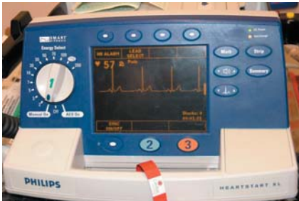
Figure 7: A cardioversion machine (panel A) which is connected to the patient via patch electrodes (panel B) positioned on the front of the chest.
